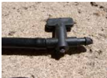
Valve connected to 1/4-inch tubing
