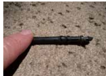
Coupler inserted in 1/4-inch tubing
