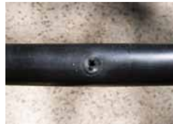
Hole punched in tubing
